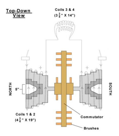
The steel core is now all one piece. It does not move. The disc has bearings in its hub that allow it to spin freely upon it. It is made of insulated copper pieces and has a lip for the brushes that would normally touch the axis. There are a series of brushes along the equator. It is said that the output is such that one can draw 4 or more currents off of it simultaneously.
