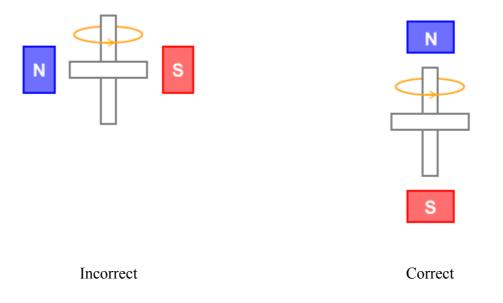
We can turn our coil arrangement into a type of brushed DC motor-generator by mounting a disc between them and using the steel core as a shaft. It is similar to a Faraday Disc in overall layout.
